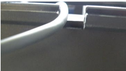
Rain-protected cable aperture at case open (IP43 configuration)
