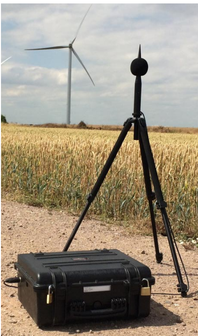
IP65 Heavy Duty Outdoor Case with pad locks and outdoor mic mounted on tripod
