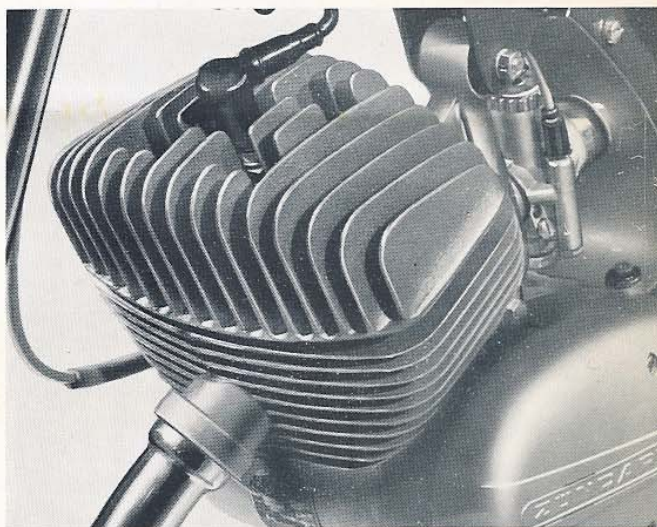
The robust, high-performance 100 c. c. two-stroke engine achieves 9.0 h. p.
