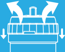
DEPRESSING THE VALVE CAP AGAINST THE SPRING RELEASES THE VACUUM
