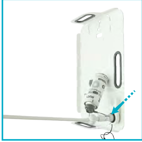
5. LUBRICATE THE MAGNIFIER LAMP SOCKET IN THE LIGHT BRACKET REGULARLY WITH RUCK MAINTENANCE FLUID (art. no. 10353).
