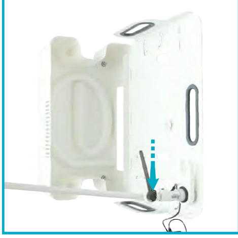
7. READJUST LAMP HINGES. FOR THIS, REMOVE JOINT CAP AND SECURE WITH OPEN-END WRENCH (INCLUDED IN THE SCOPE OF DELIVERY OF THE LIGHTS).
