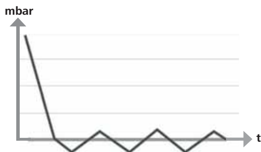
Schematic view of two-position vacuum control
