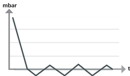
Schematic view of two-position vacuum control
