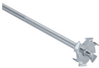
R 1303 Dissolver stirrer Radial flow, for drawing the material to be mixed from the top and bottom. High turbulence, high shearing forces. Particle reduction. Used at medium to high speeds. Ident. No. 0002746700
