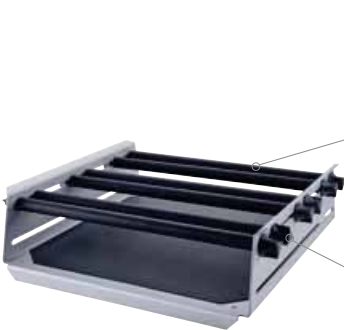
AS 4000.1 UNIVERSAL ATTACHMENT For use with various types of vessels. Infinitely variable clamping rolls allow universal adaptation to the vessels. Included with delivery: 1 x Basic holder, 6 x Clamping roll, 12 x Fastening screw
