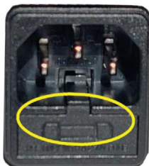
Fig. 84 - Shutter with fuses to remove
