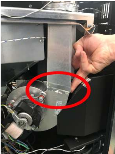
Fig. 47 - Seal with adhesive aluminium tape
