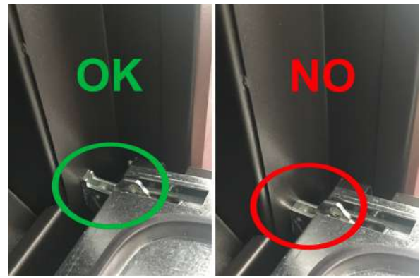
Fig. 73 - Correct hooking of the hinge
