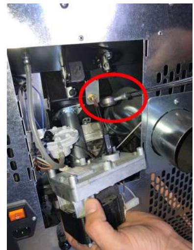
Fig. 93 - Gear motor removal
