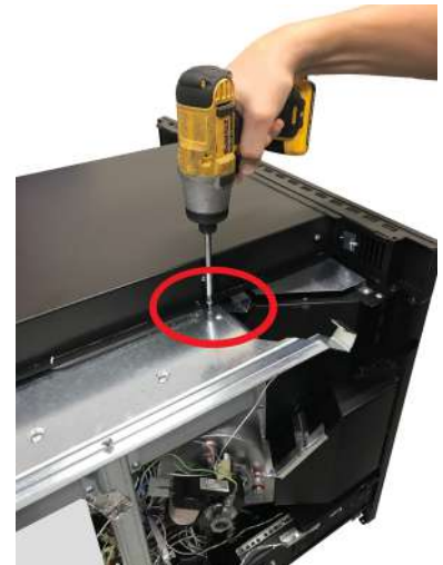
Fig. 58 - Drawer central fixing
