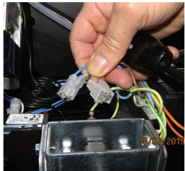
Fig. 89 - Double faston connection
