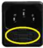
Fig. 118 - Shutter with fuses to remove
