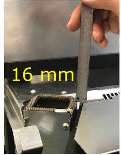
Fig. 46 - Projection of the air diverter
