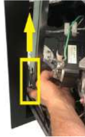
Fig. 22 - Lift locking plate
