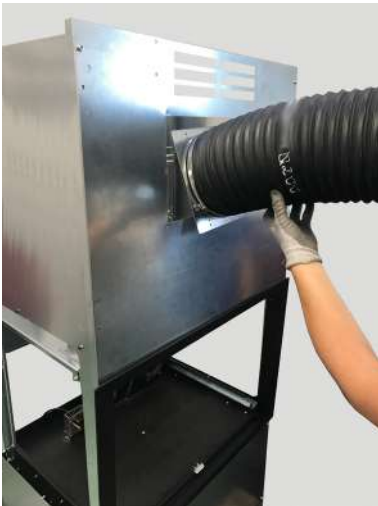
Fig. 67 - Flexible hose positioning
