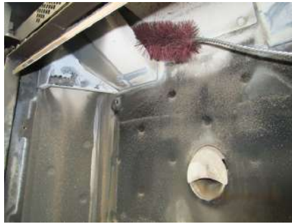
Fig. 113 - Cleaning with pipe cleaner
