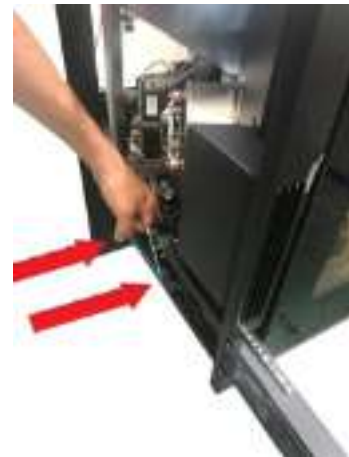
Fig. 24 - Machine body removal
