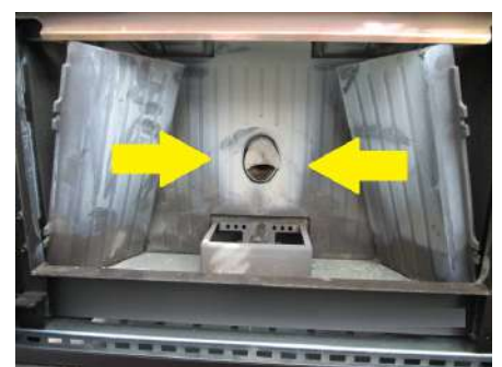
Fig. 111 - Side cast iron removal
