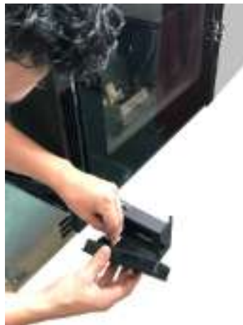
Fig. 82 - Remove the flat cable
