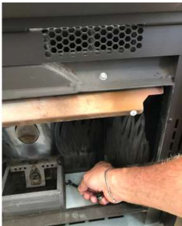
Fig. 102 - Remove the screws
