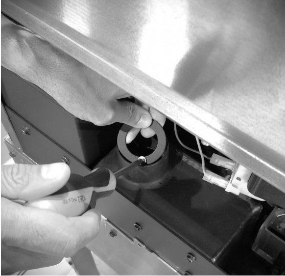
Fig. 79 - Remove the ring
