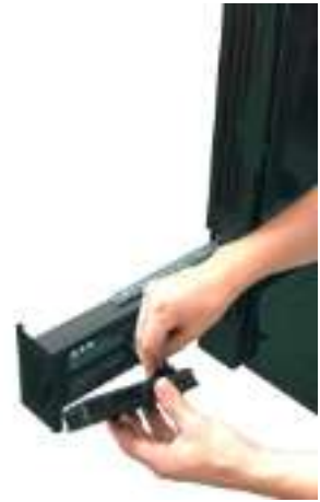
Fig. 86 - Connect and reposition the display
