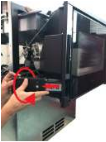
Fig. 84 - Rotate the display box
