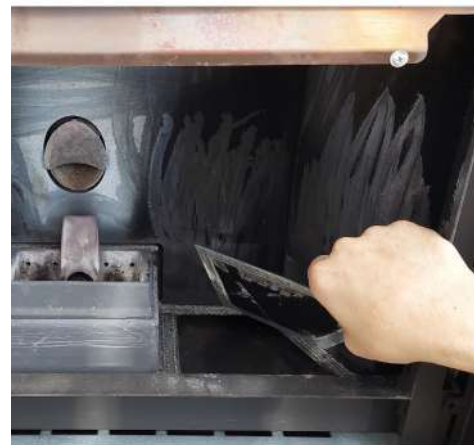
Fig. 103 - Remove the inspection cap
