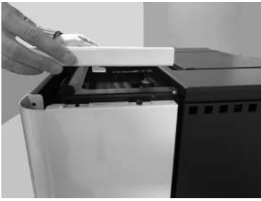
Fig. 23 - Placing the top panel
