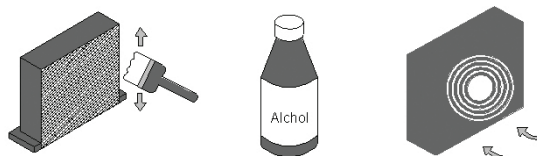
Figure 6 Cleaning of the Condenser
