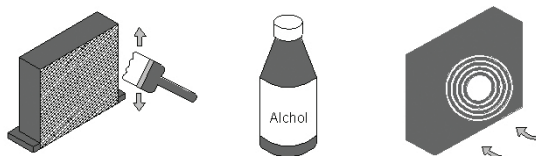
Figure 6 Cleaning of the Condenser
