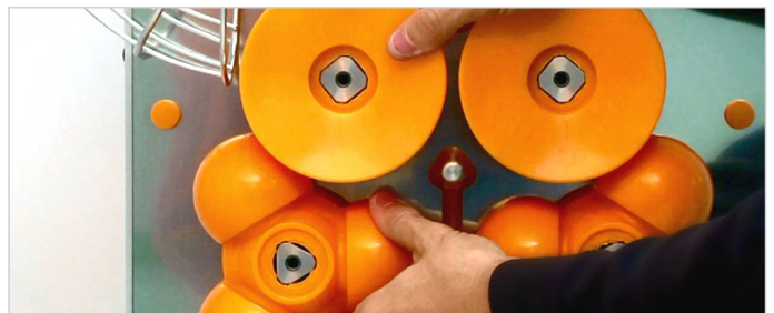
8. Take off the pressing units in pairs.
