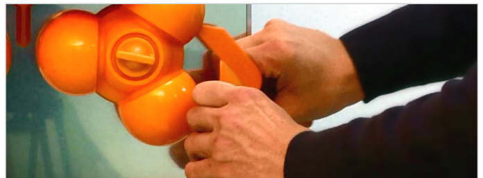
6. Pull off the peel ejectors.
