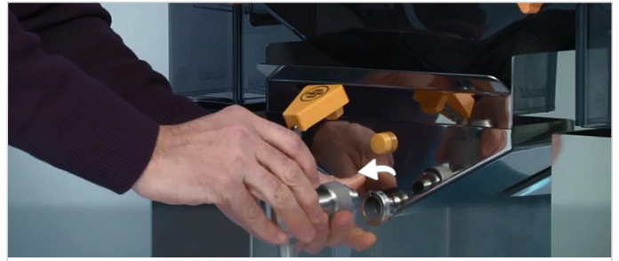
2. Remove the Self-Service tap.
