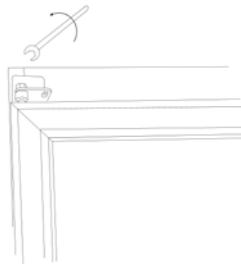
8. Tighten the top hinge pin.
