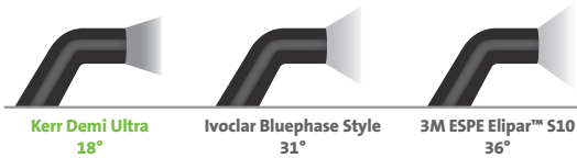
Collimation as measured by the angle of beam divergence.
