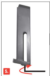
5. Turn the piercing screw upwards, pierce CO 2 -capsule.
