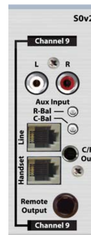
Fig 2-8: Channel 9 Rear Panel Connectors.
