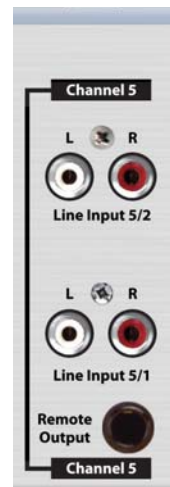
Fig 2-5: Channel 5 Rear Panel Connectors.
