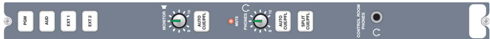
S2-OMC Control Room Monitor Channel.
