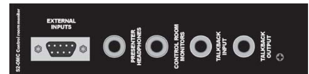
S2-OMC Control Room Monitor Rear.
