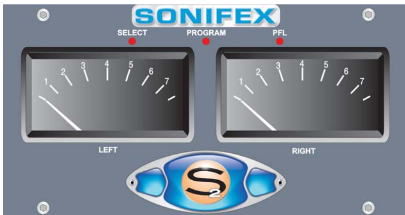
Fig 20-4 : PPM & True PPM Meter Panel.
