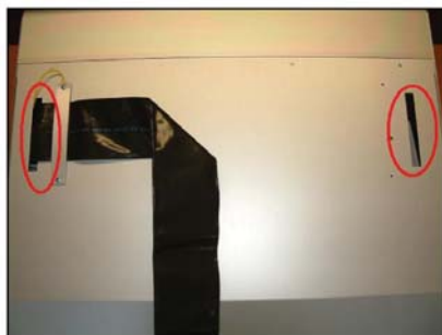
Fig 2-13 : Mixer Bus Cable Slots.
