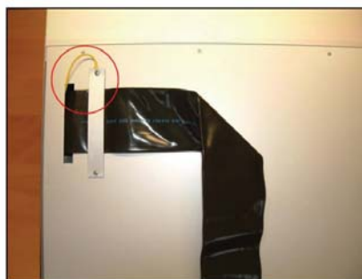
Fig 2-14 : Mixer Bus Cable Screen Connection.
