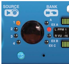
Fig 1-6: RM-2S4 Source Selector
