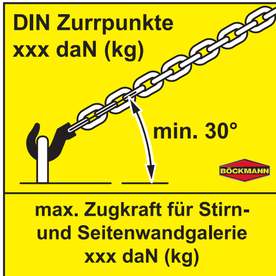
Fig. 11: Lashing points on the trailer
