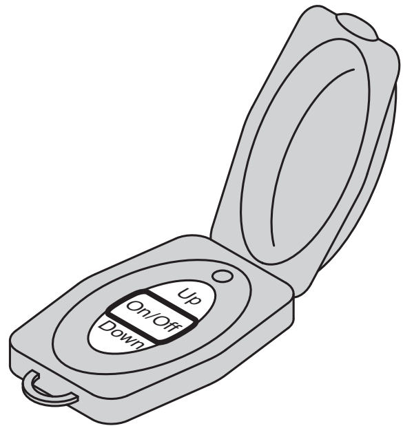
Fig. 56: Remote control for electrohydraulic pumps
