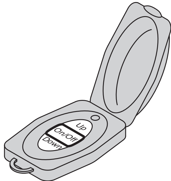
Fig. 60: Remote control for electrohydraulic pumps
