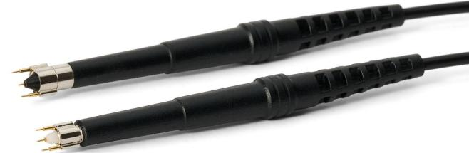
The dual ground options, a dual needle ground with a 2.3mm tip pitch, perfect for PCB-mounted RF connectors, and a solid single ground with a 6.5mm tip pitch, designed for when ground points are farther away, make this probe adaptable to a wide variety of setups, offering flexibility no engineer should be without.
