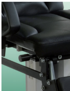
Operating handle for manual seat adjustment, shift range 150mm with 4 detents (optionally on right or left side – from user's view)
