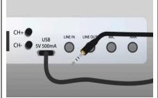
Plug in the audio cable in the "Line in" connection.
