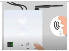
Push talk button and make your announcement when the green light is on. If you can hear the voice in the speaker, the system is installed correctly.
