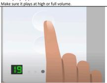
Adjust volume with the up or down button. The green display indicates selected volume.
