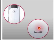
When correct phase is selected the power LED comes on and the speaker is powered.
