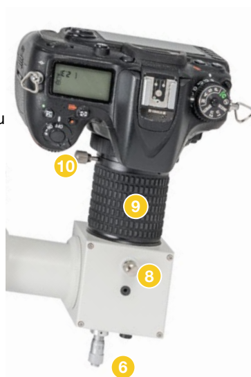
The necessary parts for focusing a camera and selecting the wavelength range, shown here with a DSLR
