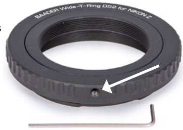
The inner thread of a T-2 ring (shown here: Baader Wide-T-Ring for Nikon Z #2408335) can be rotated into a convenient position by loosening three small setting screws.
