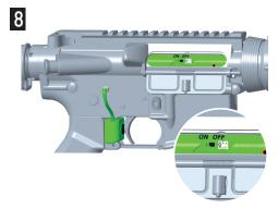
Connect the trigger switch cable with the Flash Bolt and switch main switch to "ON".
