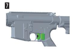
Secure the trigger switch with the magnetic trigger switch side plate.
