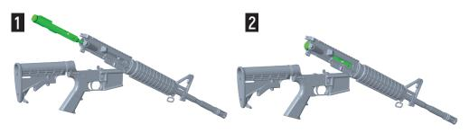
Remove original bolt carrier group from your AR. Guide the Flash Bolt into your receiver, laser tip forward.
