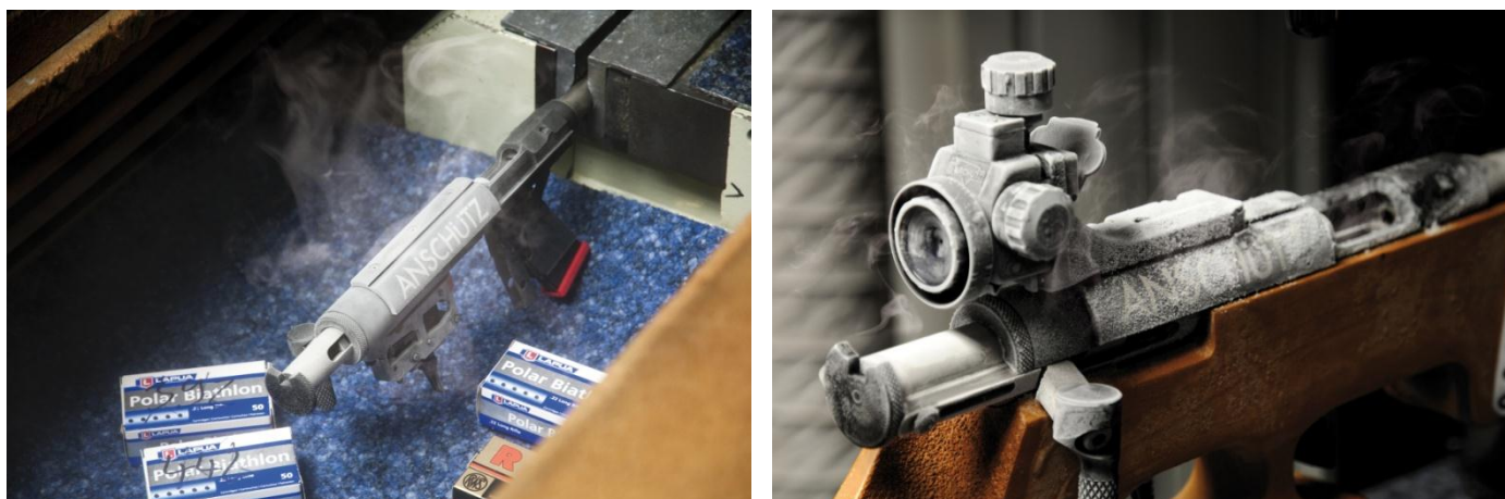
Pictures : Shooting tests in the cold chamber of company Anschütz at -30°C
