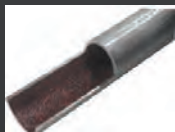
INSIDE THE PIPING OF AN OILFREE COMPRESSOR
