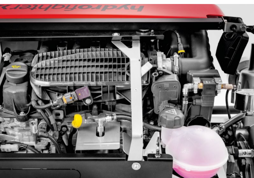
Water-cooled 3-cylinder 4-stroke gasoline engine, silent engine operation with low vibration, low flue gas temperatures
