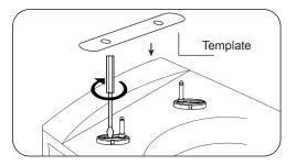
We have included a Fitting Template to make it easier to install the seat.
