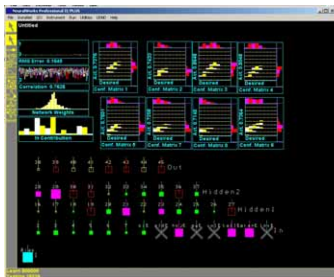
Figure 1. Screenshot of the NeuralWorks software during network training. The network structure is shown in the lower part with 14 input nodes in the input layer, 12 and 10 nodes in the two hidden layers and 8 output nodes representing estimated forest parameters. In this example, input nodes representing age, basal area, stem volume and broadleaf proportion are disabled. Scatter plots show the correspondence between actual and estimated values for the evaluation data set.
