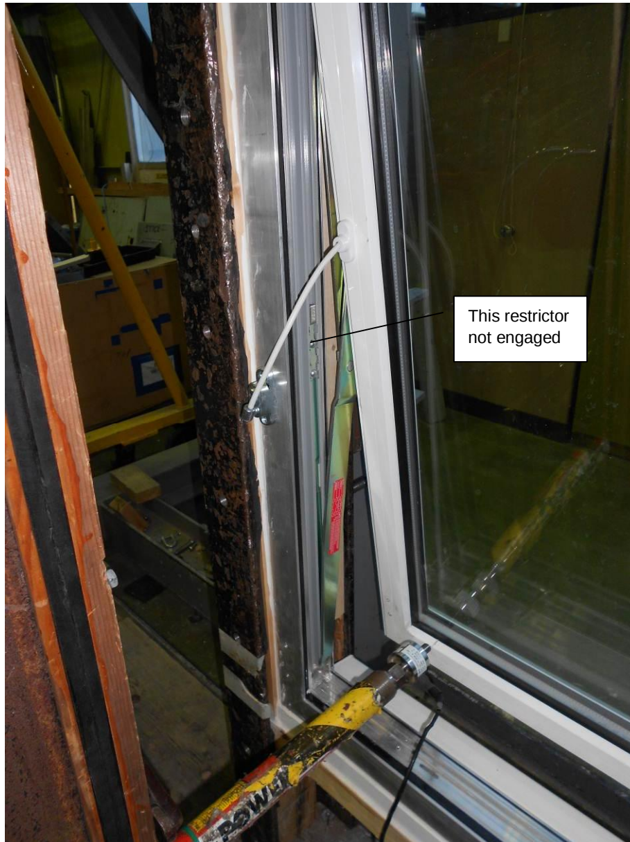
Figure A4. Penkid window restrictor under test – mounted higher up the frame, loads applied at bottom of window.
