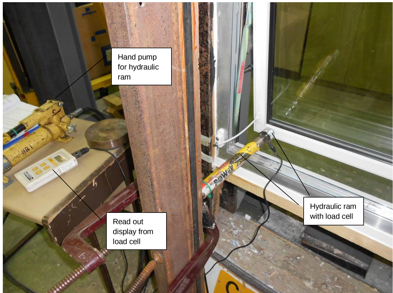
Figure A3. Penkid window restrictor under test.
