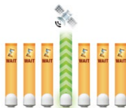
Fixed-assignment TDMA VSAT systems divide bandwidth into time slots, forcing users to wait their turn.
