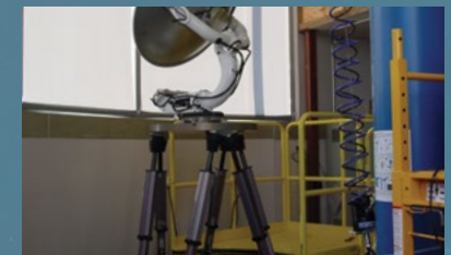
KVH Testing Facility with Hexapod Motion Table
