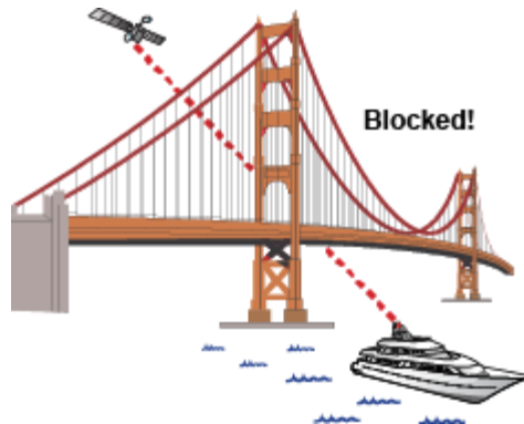
Figure 2-2 Example of Satellite Blockage
