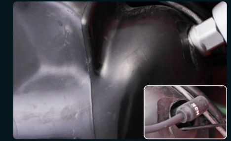
13: Screw in new spark plug. Renew spark plug connector if necessary. [SIP art.-no. see pages 18 & 19].
