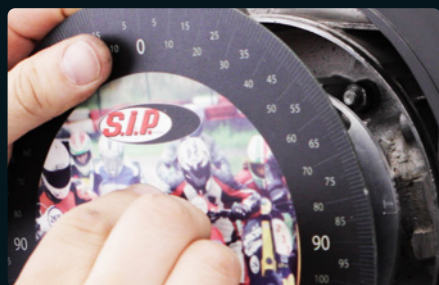
07: Align degree disc in this position with indicator to zero position. Do not turn the rotor!
