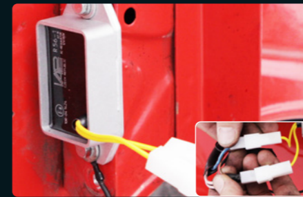
14: Mount regulator. Connect with enclosed plugs. Replace all lamps to 12V. Countercheck timing with a strobe gun!
