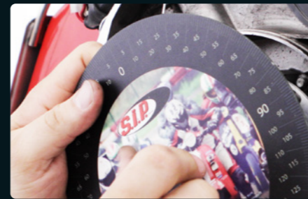
06: Place degree disc and indicator [SIP art.-No. 83002300]. Rotate rotor clockwise against piston stop tool.
