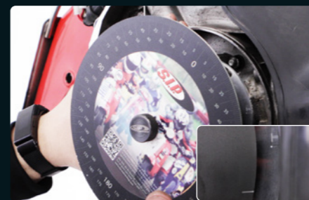
09: To calculate top dead centre [TDC] divide in half your measured value. Remove piston stopper. Turn the rotor exactly to the determined value. [Example: 43°]
