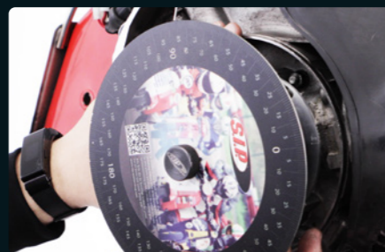
08: Rotate rotor counterclockwise together with locked degree disc against piston stop tool. [Example: 86°]
