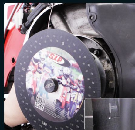
10: Rotate rotor counterclockwise together with locked degree disc and align disc / indicator with your calculated value. Keep rotating counterclockwise until T-mark on ignition base plate aligns with laser mark on rotor. Read out angle degree. [Example: 23°]
