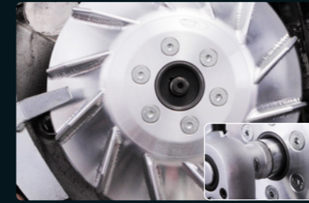
12: Mount holding tool. Mount the rotor with nut and star washer on the crankshaft. Tighten fly wheel to 45-60 Nm. [SIP art.-no. see pages 18 & 19].
