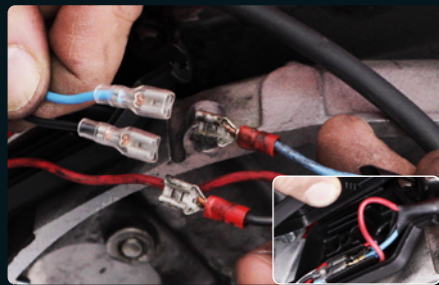
04: Check connectors. Replace if necessary [enclosed]. Pay attention to matching colours! [SIP art.-no. see pages 18 & 19].
