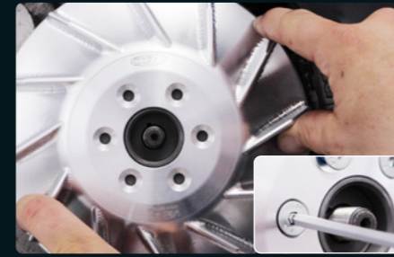
11: Mount fan wheel and align with rotor. Insert enclosed screws with Loctite. Torque: 12-14 Nm. [SIP art.-no. see pages 18 & 19].
