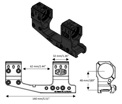
The mounts are machined from billet 7000-series aluminum and all aluminum parts are hardcoat anodized. The Torx 20 ring and clamping screws are zinc-nickel coated for corrosion resistance and come pre-waxed from the factory to ensure proper torque values.
