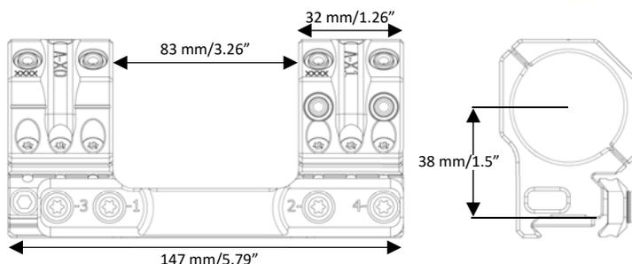
The mounts are machined from billet 7075 T651 aluminum and all aluminum parts are hardcoat anodized. The Torx 20 ring and clamping screws are zinc-nickel coated for corrosion resistance. The screws come pre-waxed from the factory to ensure proper torque values.
