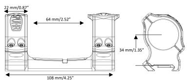
The SCP-4006D Interface Mount features two Spuhr Interface™ Top Covers, which can be installed as to position any of more than 40 different accessories in either the 12 or 3 o'clock position.
