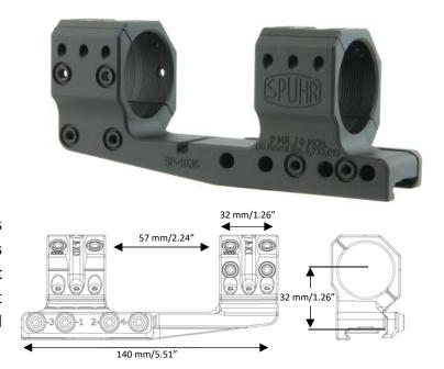
The mounts are machined from billet 7075 T651 aluminum and all aluminum parts are hardcoat anodized. The Torx 20 ring and clamping screws are zinc-nickel coated for corrosion resistance. The screws come pre-waxed from the factory to ensure proper torque values.
