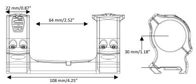
The SCP-3001 Hunting Mount features one Spuhr Interface™ Top Cover, which can be installed as to position any of more than 40 different accessories in either the 12 or 3 o'clock position.
