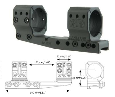
The mounts are machined from billet 7075 T651 aluminum and all aluminum parts are hardcoat anodized. The Torx 20 ring and clamping screws are zinc-nickel coated for corrosion resistance. The screws come pre-waxed from the factory to ensure proper torque values.
