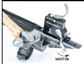
4a) Insert the trigger assembly and gently tap the front trigger pin in, from right to left. Ensure that the pin is not contacting the bolt release as this can jam the bolt catch, which is dangerous.
