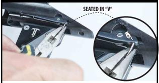
5a) If you have a bolt catch, adjust the bolt release to the bolt catch by using a pair of narrow pliers and gently bend the tab until it slots perfectly into the bolt catch notch. At rest, the bolt release should be seated in the "V", as shown. This may take several attempts.
