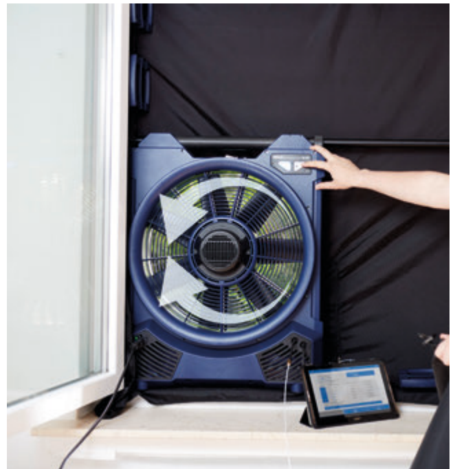
Standard-compliant Blower Door Measurement Measuring method according to ISO 9972, EN 13829 and common country-specific standards. Under- and overpressure measurement with flow rates up to 6000 m³/h without having to turn the fan unit.
