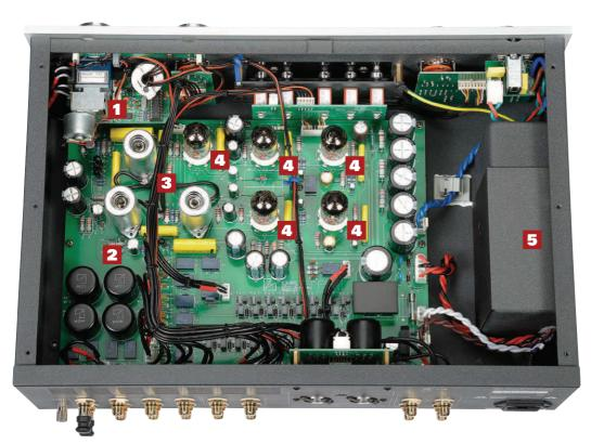
The volume control in the preamplifier is done traditionally via a, here, motor-driven potentiometer 1. In the Phono-MC stage. two pairs of transformers switchable from the front panel 2 raise the currents for the following tubes 3, which are shielded against interference. The main amplifier consists of five double triodes of type ECC82 4. The mains transformer 5 is encapsulated to protect against interference.
