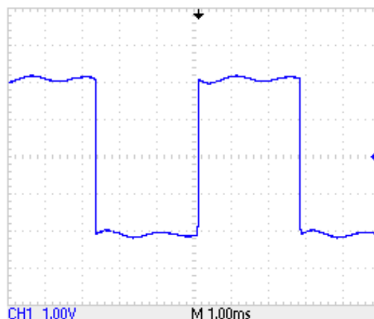
F7 SQUARE WAVE INTO 1MH + 50 UF SERIES LOAD RIGHT = WITH POSITIVE CURRENT FEEDBACK
