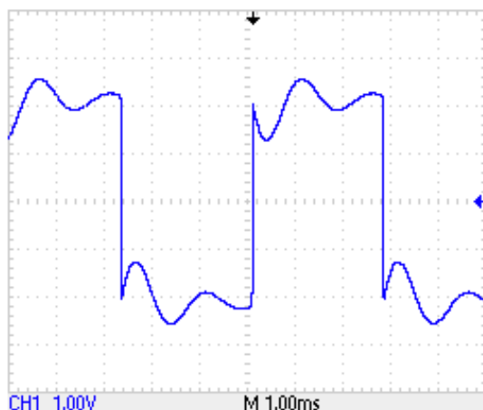
F7 SQUARE WAVE INTO 1MH + 50 UF SERIES LOAD RIGHT = WITH POSITIVE CURRENT FEEDBACK
