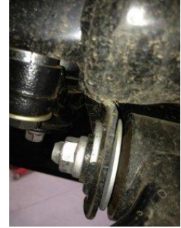
6mm spacer installed into diff mount under passenger side of vehicle (side view)
