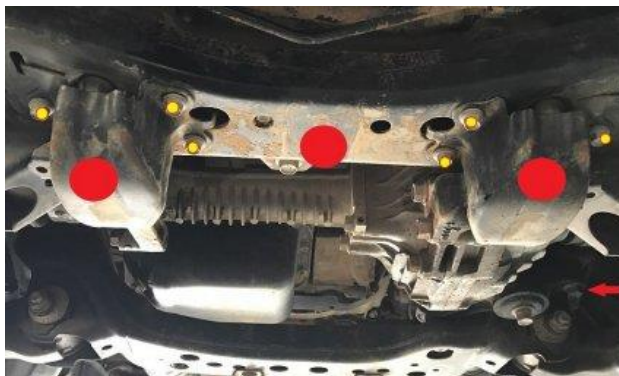
Red dot indicates the larger main diff drop spacers and bash plate mount, inc. new bolts. Yellow dots are the small spacers with new bolts. Red arrow locates the 6mm spacer.
