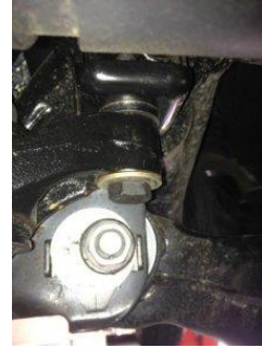
6mm spacer installed into diff mount under passenger side of vehicle
