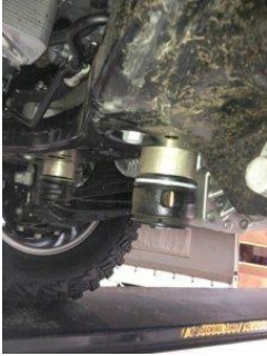
Shows Two Main Spacers Installed from rear view
