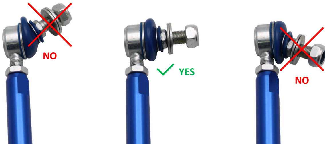
Figure 1 - Sway bar link ball end positions
