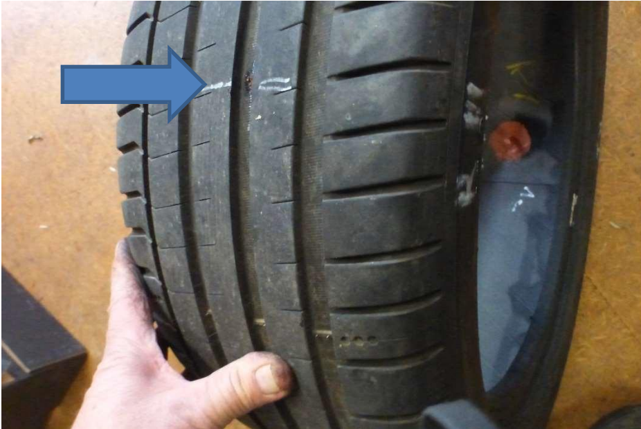
Repair points on tyres 2. The repair point is visible approx. 180° from the Repair site 4
