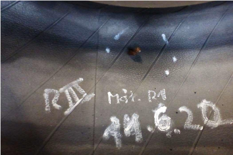
In the case of tire II, the hole channel of repair 1 was installed in the tread and a diameter of approx. 5mm. The repair site was positioned in the outermost repairable area of the tread.
