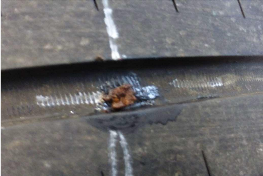
Repair point in the tread base of tyre 1 approx. 180° opposite repair point 1 Material Manufacturing date is given as 12.05 2022
