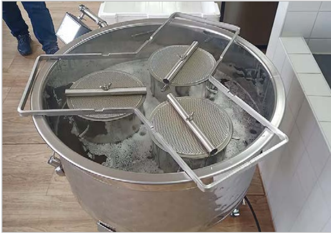
Braumeister with frame for hanging the malt pipes.
