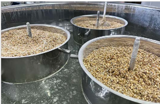
Braumeister 100 litre with three malt pipes
