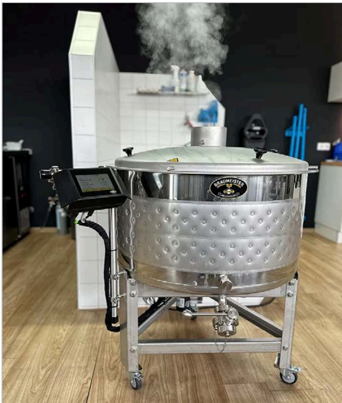
Boiling process with the Braumeister 100 litres.
