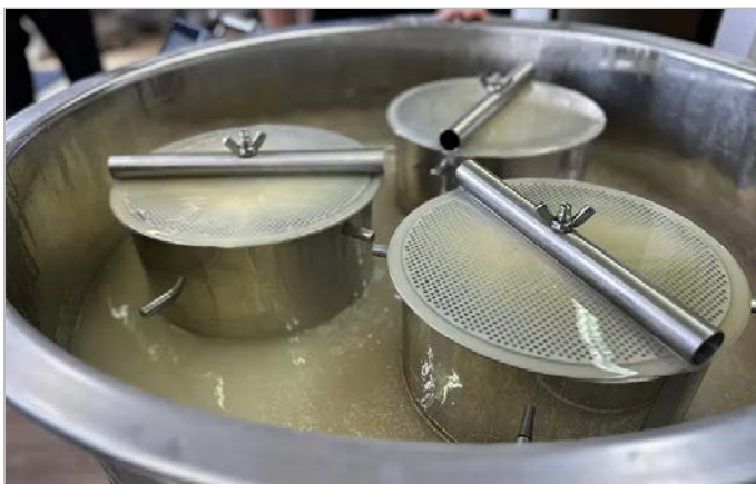
Braumeister 100 litre with attached sieve plates
