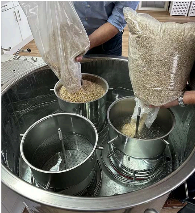
Mashing of the Braumeister 100 litre, the inserted sieve plate can be seen on the left.
